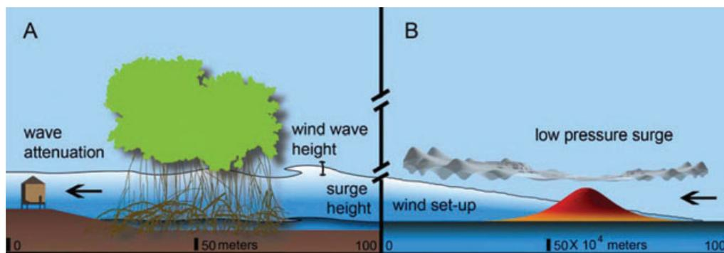
**Figure 2** (A) While vegetation may be able to dampen wind waves that pass in a period of seconds and have a wavelength measureable in meters, it cannot stop storm surges which are often on the scale of  $10^5$ – $10^6$  m in wavelength, and take several hours to inundate an area. A storm surge behaves more like tidal forces, able to penetrate diffuse vegetation
